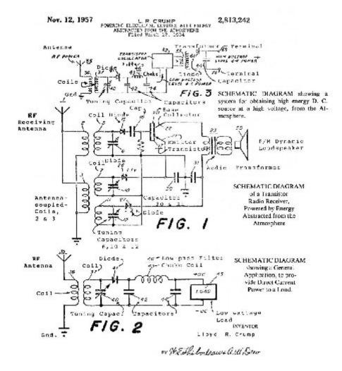
Coil and capacitor are tuned to frequency of a radio transmitter from which the diode rectifies the signal and delivers a D.C. pulsating current , a full wave rectifier would give a better output.
